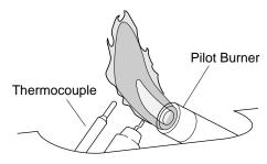
Figure 20 - Incorrect Pilot Flame Pattern
